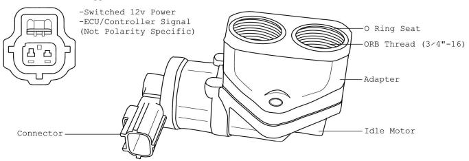
Note: For best response, inner ORB port closest to connector to intercooler pipe, airbox or atmosphere. ORB port furthest from connector to inlet manifold/plenum.
